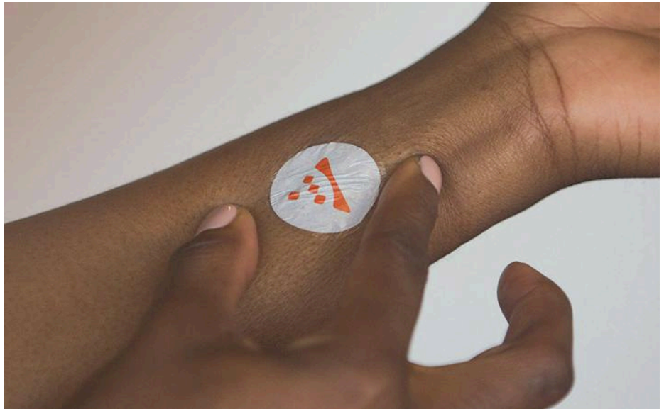
MC10’s electronic “tattoos” consist of an antenna and thinned near-field communication chip mounted onto a stretchable adhesive. (Image courtesy of MC10)
