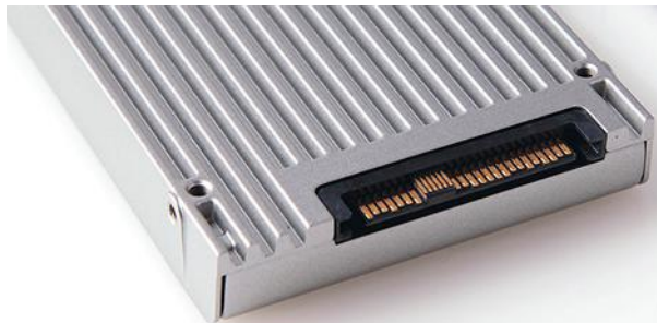
1. The U.2 connector, formally known as SFF-8639, supports up to four SAS/SATA interfaces and PCI Express x4, including dual port configurations.
