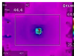
Figure 4. LTM4632 Thermal Performance. 12V Input, 3A. (Figure 2 Design)
